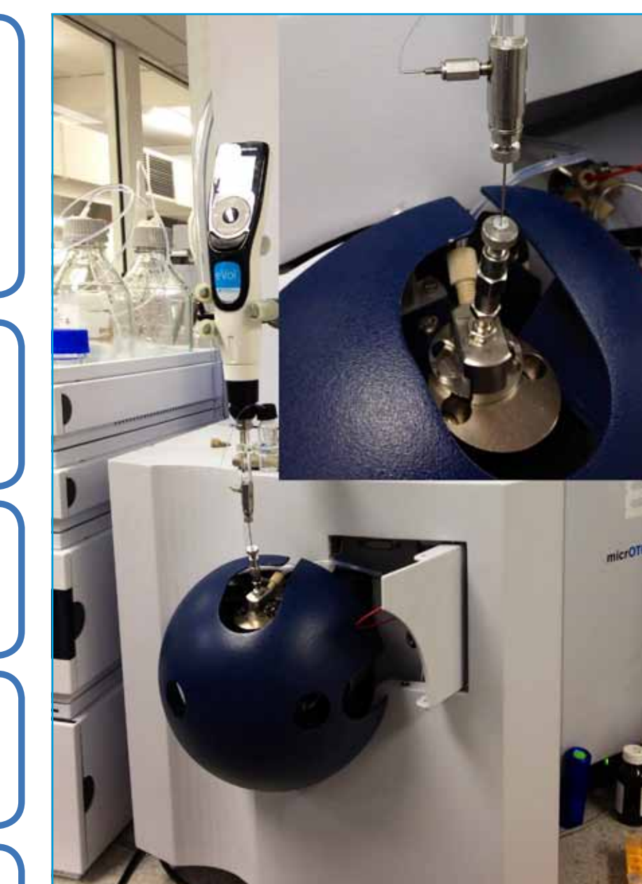
Figure 6. eVol® MEPS™ infusing directly into the ESI source.
